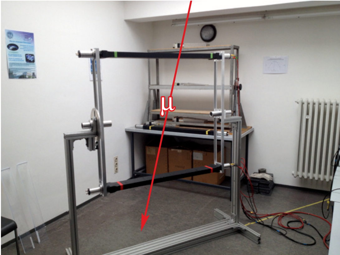
Figure 2: The experimental setup consisting of two plastic scintillators mounted in a rotatable frame. In addition, a sketch of a possible muon trajectory is shown.
