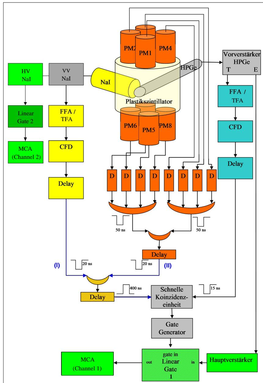
Figure 5: Schematic circuit diagram of the Anti-Compton spectrometer setup
