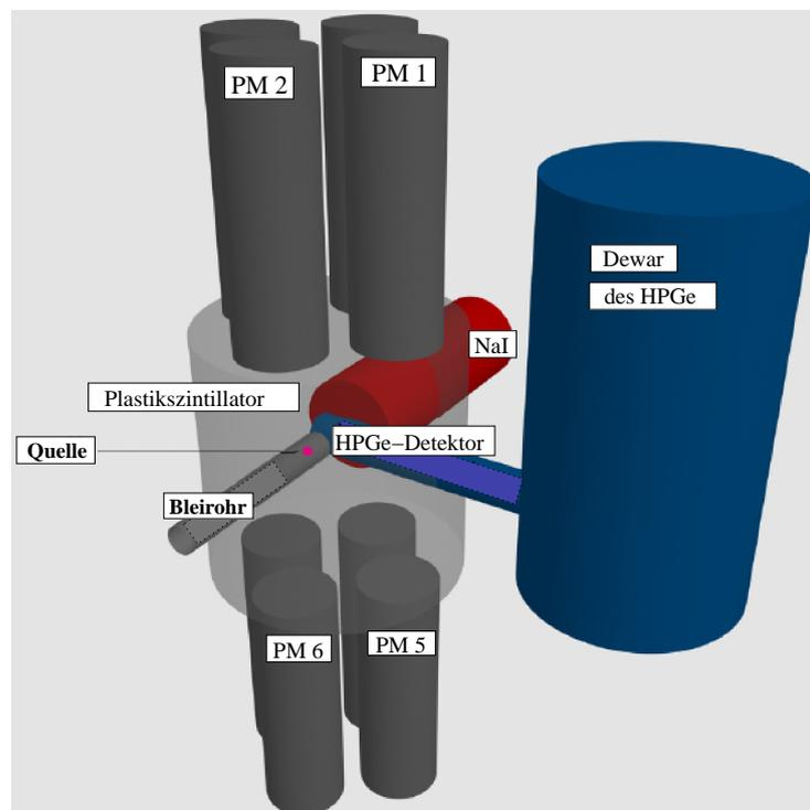
*Figure 1: Schematic figure of practical setup.*
