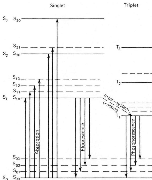
**Figure 2:** Energy levels of organic molecule with  $\pi$ -electronic structure
