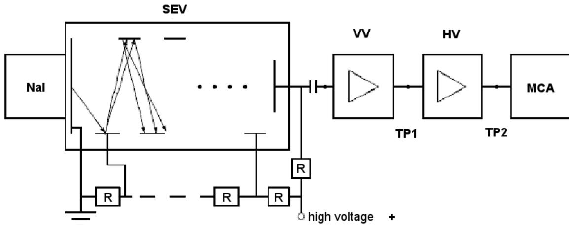
**Figure 4:** Electronic block diagram of a NaI-spectrometer,
