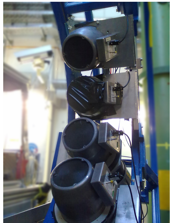
Figure 3.11: Photograph of EUROBALL Cluster detectors (left) and HECTOR (right), taken during the described S377 experiment.
